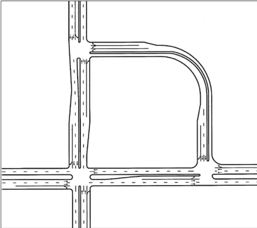
Figure 4-6: Left Turn Movements at Quadrant Roadway Intersections
