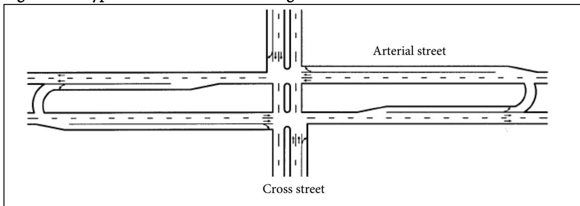
**Figure 4-3: Left Turn Movements at a Median U-Turn Intersection**
