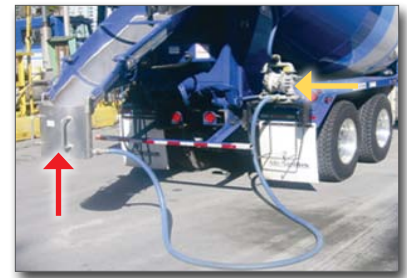
Figure 8. Chute washout bucket and pump
